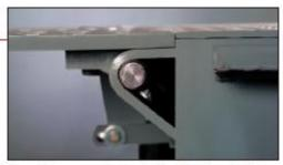
Two-point crown control on the front lip hinge distributes the load evenly, smoothes out the transition between the leveler and the trailer bed, and extends the hinge life.
